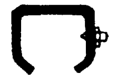
Connecting bracket #54.234 for rail #7 With set screws
