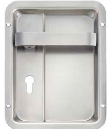
#53.5072 flush plate with lever pocket door function 244.4 x 183 mm Build in space depth flush plate: 20 mm; proud: 7 mm
