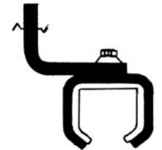
No. 8 wall bracket 54.825 sideways adjustable two parts
